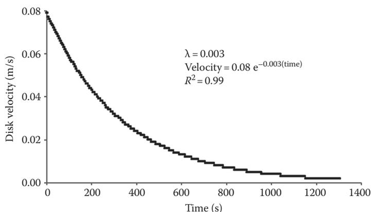
**FIGURE 10.2** Exponential decay of disk sliding velocity as a function of time. The decay rate ( $\lambda$ ) was 0.003, and initial and final disk velocities were kept at 80 and 2 mm/s, respectively.
