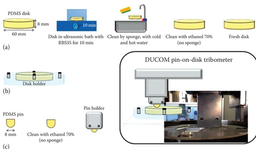
**FIGURE 10.1** Cleaning and mounting of pin-and-disk specimens for friction measurements of cow milk fat: (a) disk cleaning (left to right), (b) disk mounting, and (c) pin mounting (left to right).
