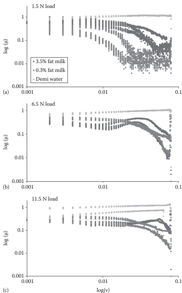
**FIGURE 10.3** Change in the friction coefficient ( $\mu$ ) as a function of disk velocity for 3.5% fat milk, 0.3% fat milk, and control (water) at normal load of 1.5 N (a), 6.5 N (b), and 11.5 N (c). Data presented include two repetitions per load. The velocity decay rate ( $\lambda$ ) was fixed at 0.003.
