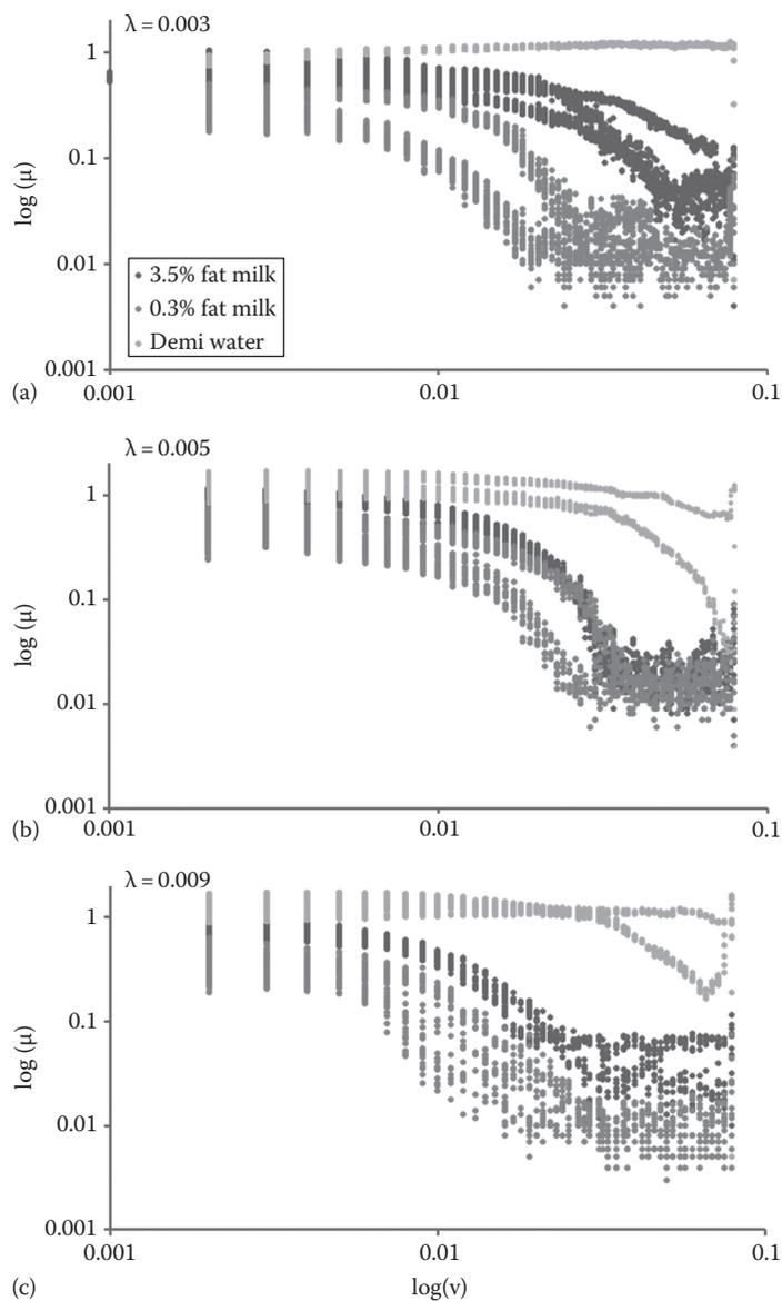
**FIGURE 10.5** Change in the friction coefficient as a function of disk velocity for 3.5% fat milk, 0.3% fat milk, and control (water) at a velocity decay rate of 0.003 (a), 0.005 (b), and 0.009 (c). The normal load was fixed at 1.5 N. Data presented include two repetitions per decay rate.
