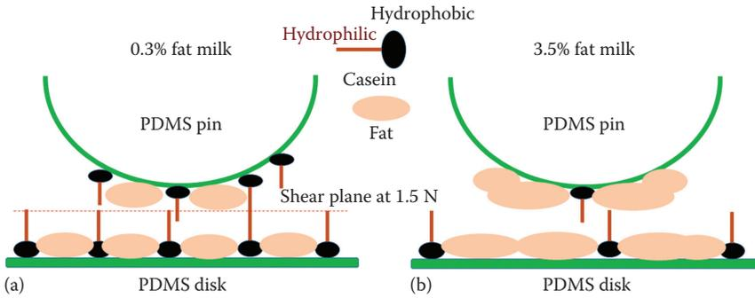
**FIGURE 10.7** Schematic of the surface layer composed of casein and fat molecules, adsorbed on PDMS surfaces after shear thinning, for 0.3% fat milk (a) and 3.5% fat milk (b).
