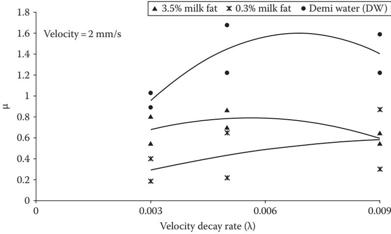
**FIGURE 10.6** Relationship between the friction coefficient at low velocity (2 mm/s) and velocity decay rates for 3.5% fat milk, 0.3% fat milk, and control (water). Data presented include two repetitions per decay rate.
