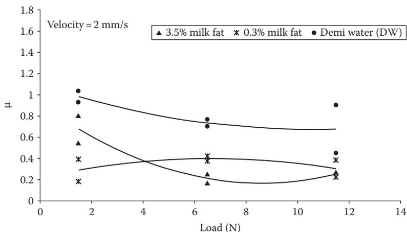
**FIGURE 10.4** Relationship between the friction coefficient at low velocity (2 mm/s) and normal load for 3.5% fat milk, 0.3% fat milk, and control (water). Data presented include two repetitions per load.
